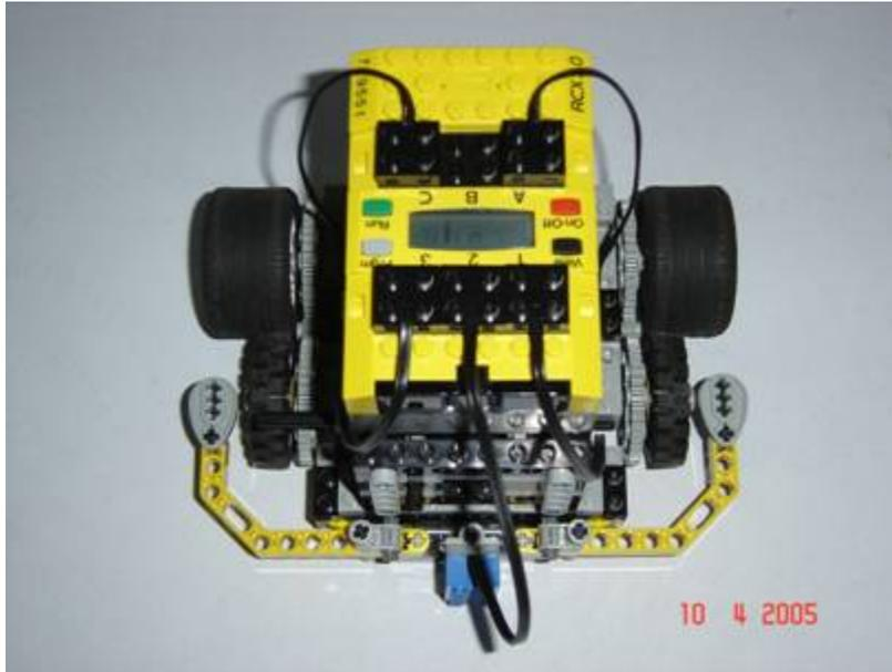
*Figure 4 - A Lego Roverbot with two touch sensors, one light sensor, and two motors*
